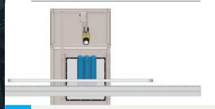
PackCheck<sup>™</sup> analyses every pack on your production line to ensure that it is complete, with no missing items and that the shrinkwrap has been correctly applied.
